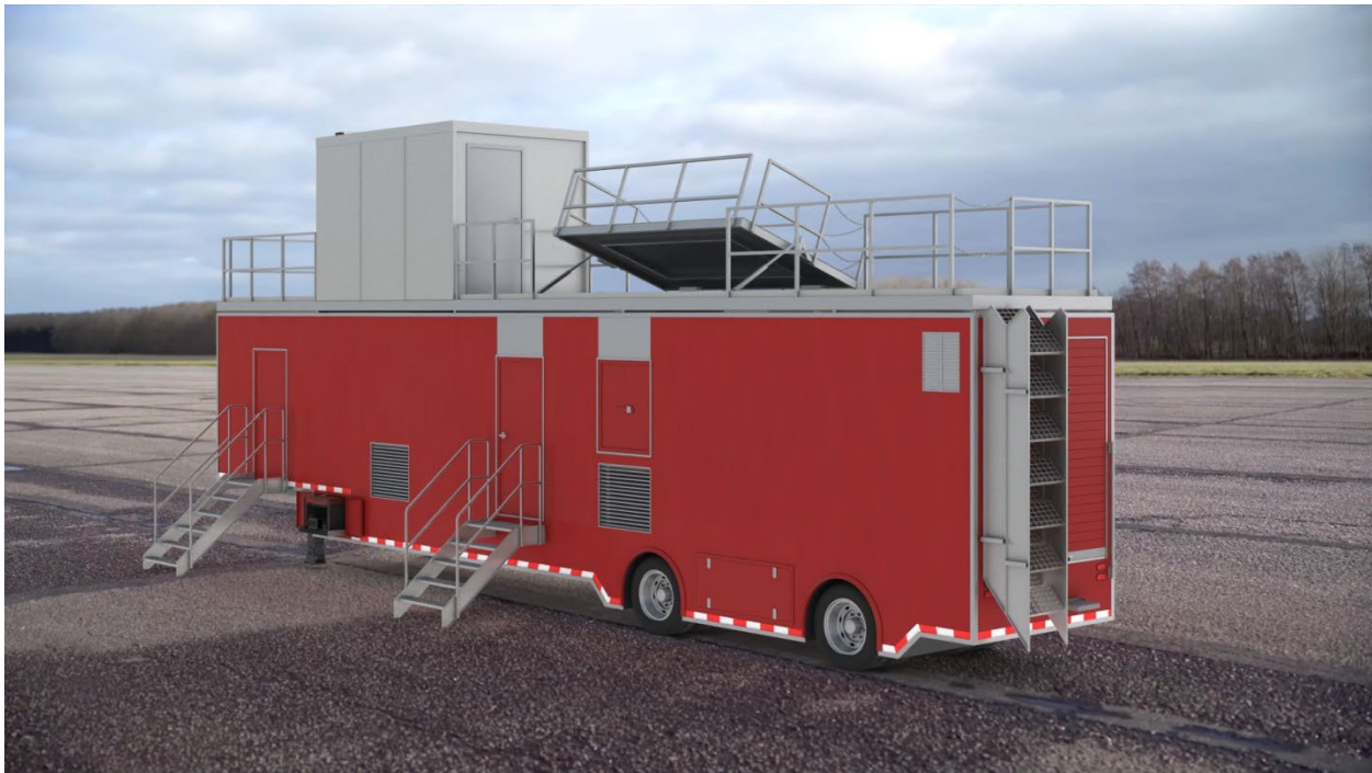
Two-Story Mobile Fire Simulator w/ Retractable 2 nd -Story Room
