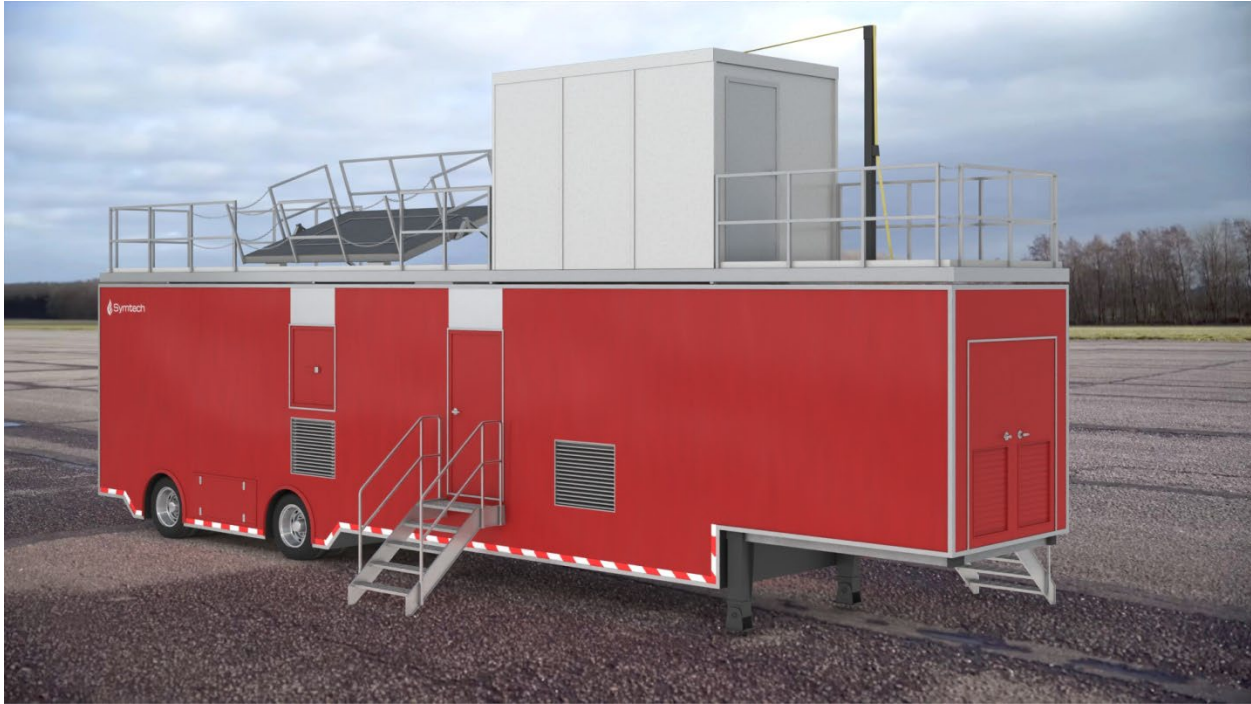
Two-Story Mobile Fire Simulator w/ Retractable 2 nd -Story Room
